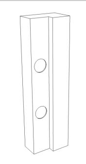
8) Using your combination square, scribe a line down either edge of this circle, and then remove the waste with either a router or a sharp chisel, referring to the below.
