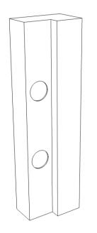
8) Using your combination square, scribe a line down either edge of this circle, and then remove the waste with either a router or a sharp chisel, referring to the below.
