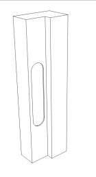
9) The next step is to chop out for the back of the keep, this is located centrally within the cut pocket, and Atlantic UK recommends that the dimensions of this pocket are 70mm high, 20mm wide and 15mm deep. This is also shown below.
